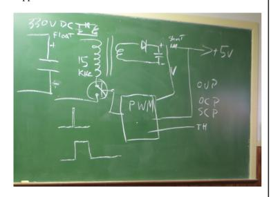
The brain behind the device above is the pulse width modulator, which can have sensors for over voltage protection (OVP), over current protection (OCP), short circuit protection (SCP) and thermal cutoff (TH).
